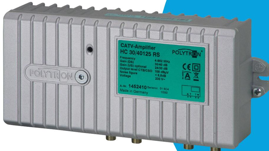
The new generation of Polytron CATV-Home-Distribution-Amplifiers – the HC series is particularly designed for the use in multiple family dwellings. The use in cable networks with multimedia (e.g. Internet) is supported by plug-in return path. The right output level can be exactly adjusted by set point bridges. The power supply guarantees a long life cycle. The housing conforms to the protection class IP 65.
