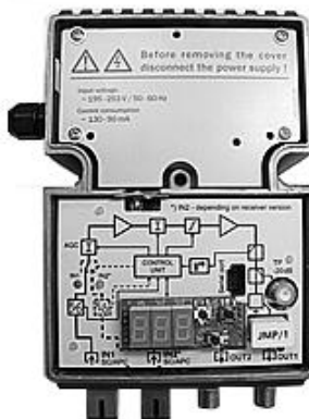
Fig. 5.1. Interior of the ORB 729 optical receiver with a TCM 729 local monitoring module.
