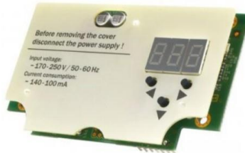
Fig. 3.6. TMM 729 remote monitoring module.
