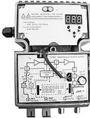
Fig. 5.2. Interior of the ORB 729 optical receiver with a TMM 729 remote monitoring module.
