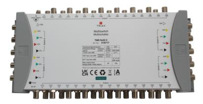
Cascade multiswitch for 2 Satellite positions with 9 inputs and 9 trunk outputs, suitable for distributing satellite and terrestrial signals in small to large sized systems. Available with 32 subscriber outputs and powered by the TMS PSU external power supply either directly or via the SAT trunk lines.
