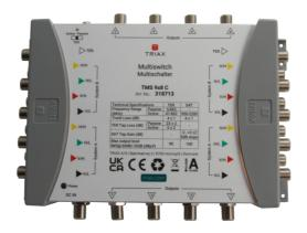
Cascade multiswitch for 2 Satellite positions with 9 inputs and 9 trunk outputs, suitable for distributing satellite and terrestrial signals in small to large sized systems. Available with 8 subscriber outputs and powered by the TMS PSU external power supply either directly or via the SAT trunk lines.
