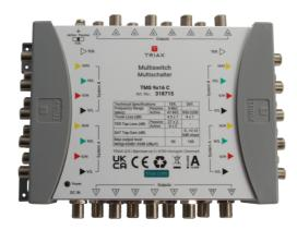
Cascade multiswitch for 2 Satellite positions with 9 inputs and 9 trunk outputs, suitable for distributing satellite and terrestrial signals in small to large sized systems. Available with 16 subscriber outputs and powered by the TMS PSU external power supply either directly or via the SAT trunk lines.
