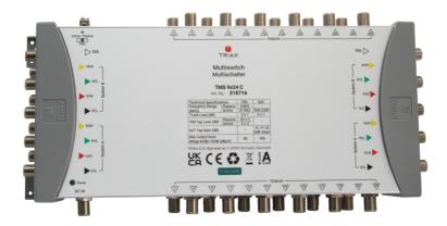
Cascade multiswitch for 2 Satellite positions with 9 inputs and 9 trunk outputs, suitable for distributing satellite and terrestrial signals in small to large sized systems. Available with 24 subscriber outputs and powered by the TMS PSU external power supply either directly or via the SAT trunk lines.
