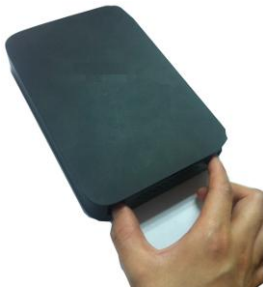
① Draw out the HDD bracket
