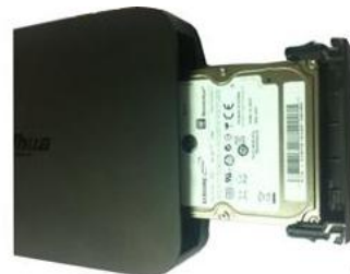
③ Put the HDD into the device
