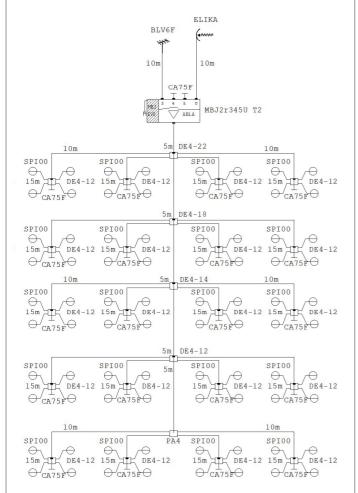
The RF output level settings are separated and stabilized by the Automatic Building Level Adjustment (A.B.L.A. circuits).
