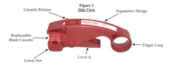
Thank you for choosing a Cablematic® tool manufactured by Ripley Tools. The proper use of this cable preparation tool will result in error free preparation of the drop cable end. In one step, both the center conductor and braid exposure lengths are prepared to SCTE and Bellcore specifications.
